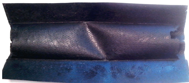
Fig. 5. Long test specimen in self-locked state
