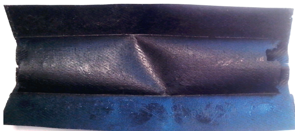
Fig. 5. Long test specimen in self-locked state
