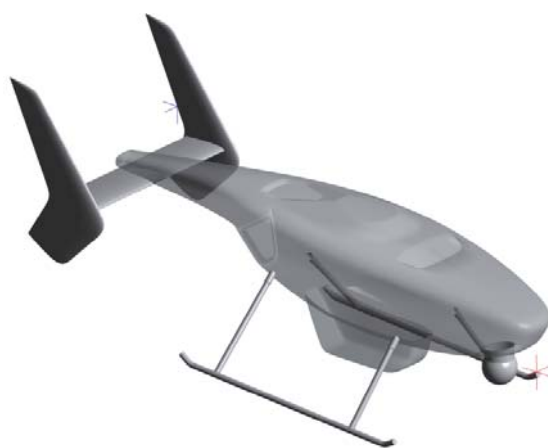
Fig. 1. The appearance of the layout of the helicopter and the position of the points P_{\min} and P_{\max} starting with the hundredth iteration (the front edge of the landing gear and the rear edge of VT)
