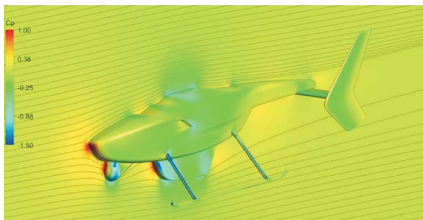
Fig. 4. Pressure coefficient C_p and streamlines in the plane of symmetry
